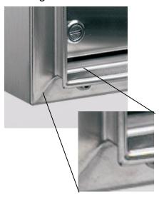
The surface of contact to the gasket is wider than conventional profiles, and has no sharp edge. This ensures that the gasket will not get cut, and will not lose its shape memory. In this way the tightness is guaranteed for much longer time (virtually for the whole life of the cabinet).
